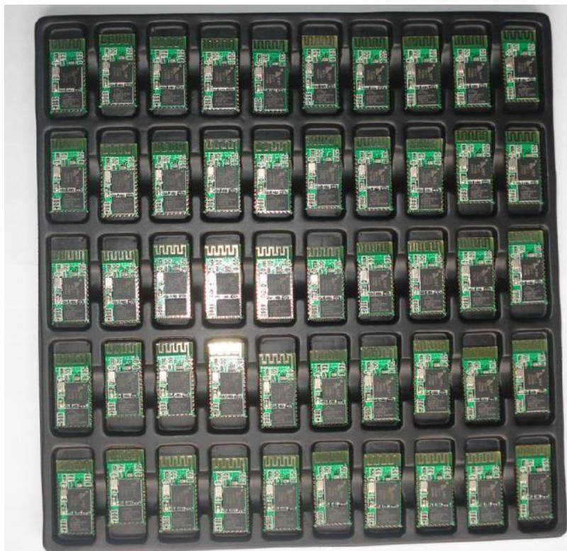
Figure 3 50 pieces chips in an anti-static blister package.
